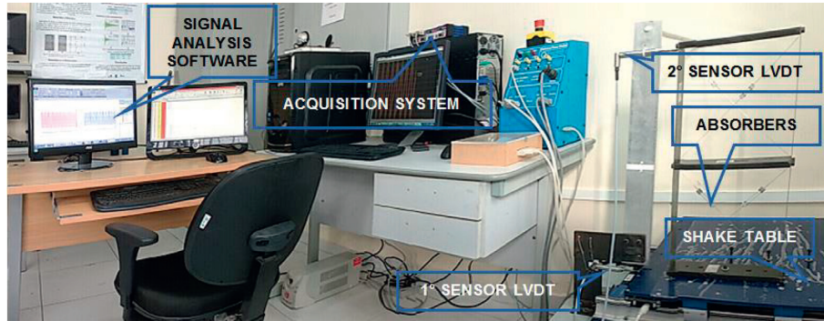
FIGURE 8: Experimental setup of the system under forced vibration.
